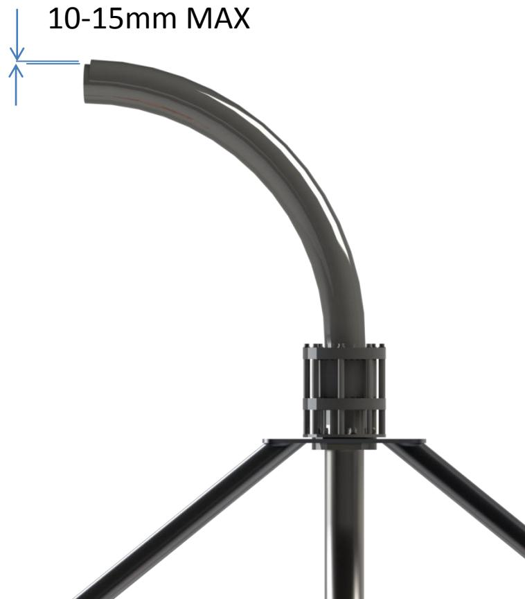
MEASURE 'PLAY' BY LIFTING THE ROTORPIPE
